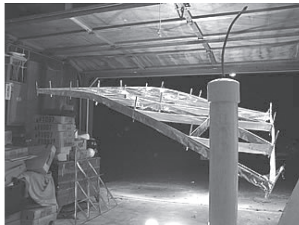
Fig. 5. Multi-Cellular Design. Multiple lifting-cells increase thrust output and overall efficiency. The Lifter-9 has 36 cells, and a combined air-gap length of 100 ft!
