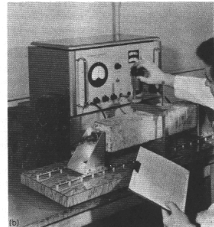
Figure 5.13 Damping capacity technique: (a) diagrammatic representation; (b) application to testing of concrete. Courtesy Dawe Instruments Ltd
