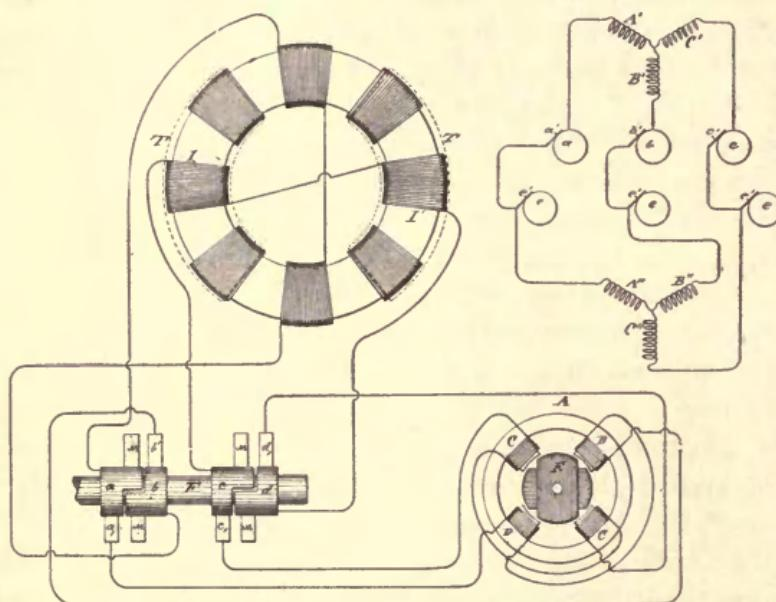
bearing on the continuous portions for taking off the alternating currents are represented by  $a'\ b'\ c'\ d'$ . The collecting brushes, or those which may be used to take off the direct current, are designated by  $m\ m$ . Two pairs of the armature coils and their commutators are shown in the figure as being utilized; but all may be utilized in a similar manner.
