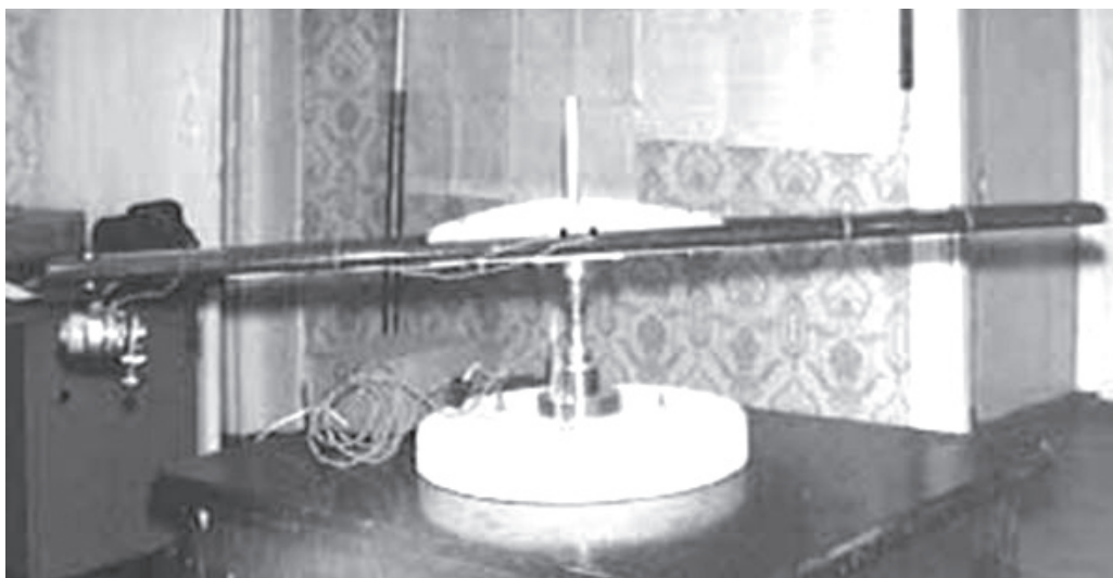
Fig. 8. “Karteziy” inertia device with small loads at the left end of the shaft; supply voltage is 12 volts.
