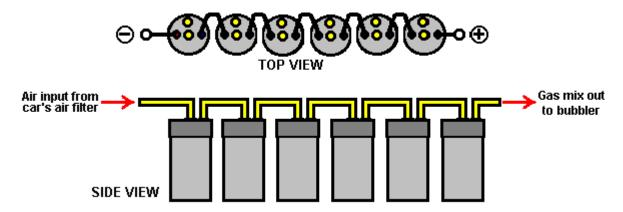
The upper diagram shows the electrical connection between the cells while the lower diagram shows how the air/gas pipes are connected. While the cells are shown side by side in the diagram, they can be positioned in any convenient locations in the engine compartment. As the temperature in the engine compartment can be quite high, the cell housings need to be unaffected by high temperatures, which make some plastic containers unsuitable for this use.
