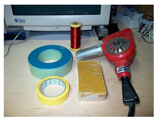
Of paramount importance with the toroid is that unlike traditional transformer design, the secondary is wound first, and the windings must be evenly spaced where they fan out from the center of the core. This means even though they are tightly packed right up against one another at the center hole, they must not be wound so that they bunch up and gap open around the periphery. Mistakes here will cause field errors that will lower the overall efficiency.
