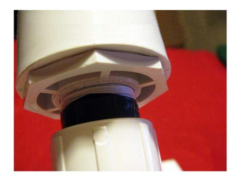
These units come with a domed cap which needs to be drilled out with a large number of 1/16" holes like this:
