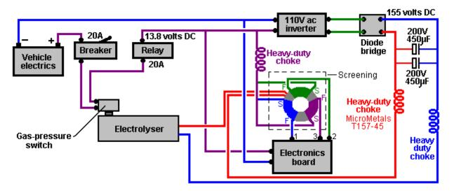
It is important to include heavy-duty chokes (coils) in both sides of the high voltage power supply and in the 13.8 volt positive lead coming from the vehicle electrics. The recommended choke cores are the MicroMetals T157-45 and these are wound with 15 turns of AWG #16 (SWG 18) enamelled copper wire, through it is perfectly ok to wind these chokes on laminated iron pieces taken from an old mains power transformer frame. The fifteen turns of wire produce a choke of 29.5 microhenrys.
