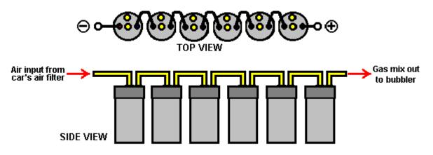
The upper diagram shows the electrical connection between the cells while the lower diagram shows how the air/gas pipes are connected. While the cells are shown side by side in the diagram, they can be positioned in any convenient locations in the engine compartment. As the temperature in the engine compartment can be quite high, the cell housings need to be unaffected by high temperatures, which make some plastic containers unsuitable for this use.
