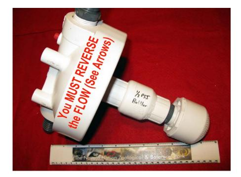
Also, the pressure at which it operates needs to be dropped from normal household water pressure to the 0.5 psi. gas pressure needed for use as a bubbler. This is achieved by replacing the ball valve inside the unit with a much weaker version available from the KBI company, reference code KC1000 and costing about US \$10. If you get one, be sure to specify a 0.5 psi pressure version as they have more than one type.
