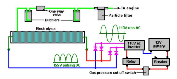
As mains voltage is quoted as an average figure ("root-mean-square") it has a peak voltage of 41% more than that. This means that the pulsing DC has a voltage peak of just over 150 volts for the nominal 110 volt AC output from the inverter.
