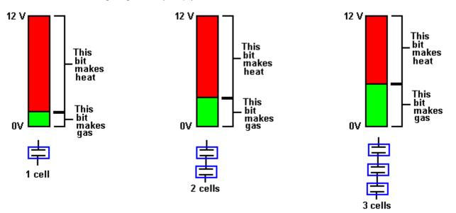
The best electrode material for the plates is 316L-grade stainless steel. It is hard to believe, but there is a voltage drop across the plate, which makes it necessary to apply about 2 volts to the plates on each side of the cell. So, if you are running off 12 volts, then six cells in a row across the battery gives the maximum possible drive. With the engine running and providing almost 14 volts, seven cells gives the highest possible drive.
