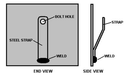
To combat splashing of the electrolyte, a layer of aquarium matting is placed over the tops of the plates. In the diagram above, only a few of the 101 plates are shown, in order to keep the drawing narrow enough to fit on the page. The plates at each end have a stainless steel strap welded to them in order to allow for simple and robust electrical connections to be made through the case.
