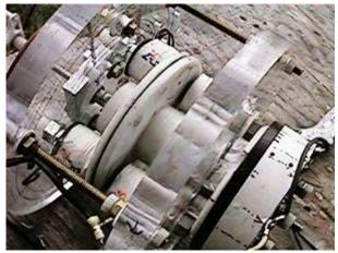
Motorcoils A and B are in parallel and switched on-off to run motor.
