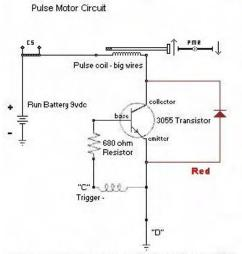
motor-coil back pulses when transistor is off
