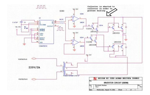
This circuit is generating a square wave of 50Hz through the 4047 IC, where the tansistors are amplifying the current. The transistors can be replaced by FETs to have lower power dissipation and faster switching. The driver circuit can be changed to have a modified sine-wave, as square wave is not good for many electric appliances.
