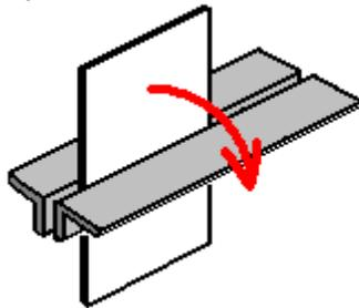
The bent sheet can then be clamped between two steel strips and a sharp U-shaped bend produced by tapping with a hammer, again, along the line of the required bend:
