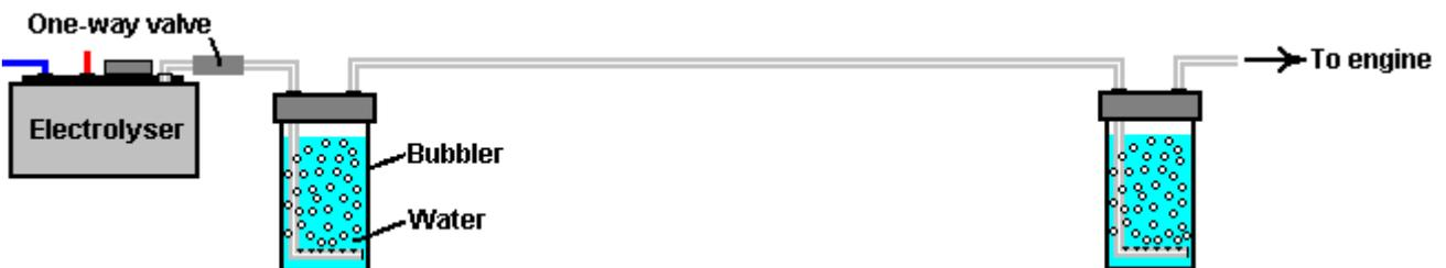
Where the first bubbler is close to the booster and the second one is placed close to the engine. Once in a while, the water from the first bubbler can be used to top up the water inside the booster so that any traces of hydroxide
