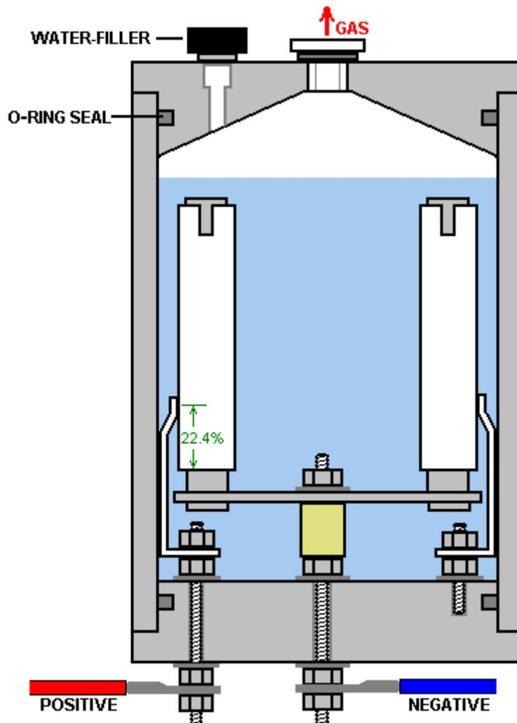
This cross-sectional view may be slightly misleading as it suggests that each of the nine outer pipes has its own separate bracket and this is probably not the case as they are connected together electrically through the steel ring-shaped disc and should vibrate as a single unit. It is tempting to use separate brackets as that would allow the assembly to be taken apart quite easily, but the electrical contacts of such a system would be much inferior and so it is not to be recommended.
