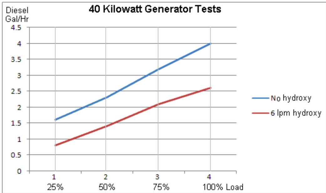
The gains at full 40 kW load are about 35%, representing a reduction of 1.4 gallons of diesel per hour. As the generator is part of the equipment of a major power supplier, it is likely that the number of generators will be manipulated in relation to the demand and so the continuous overall gain is likely to be about 33% even with such a low hydroxy input as 6 lpm. The investigation and development is continuing.
