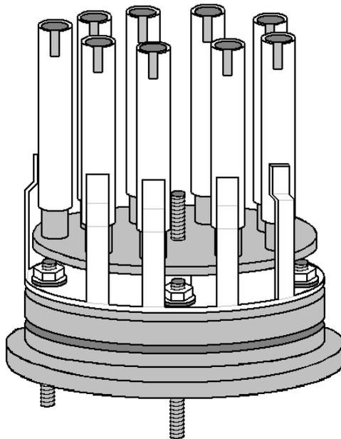
The ring support for the outer pipes is not bolted securely to the plastic base but instead it is spaced slightly above it and mounted on just the stud points. This ring is underneath the slightly smaller diameter disc which holds the inner pipes. This makes it impossible for the two components to be slid together or apart, due to the length of the
