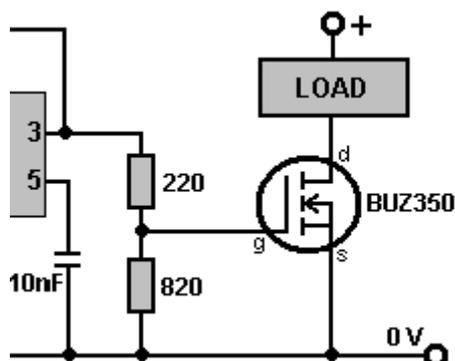
Here, the 555 chip output voltage is lowered by  $220 / 820$  or about 27%. When the voltage rises, it causes the BUZ350 transistor to switch on, short-circuiting between its Drain and Source connections and applying the whole of the 12-volt supply voltage across the load, which in our application, is the electrolyser cell:
