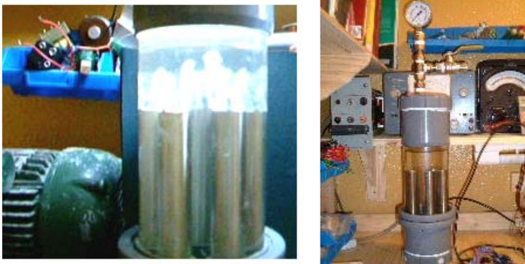
The electrolysis takes place between each of the inner and outer tubes. The picture above shows the bubbles just starting to leave the tubes after the power is switched on. The picture below shows the situation a few seconds later when the whole of the area above the tubes is so full of bubbles that it becomes completely opaque:
