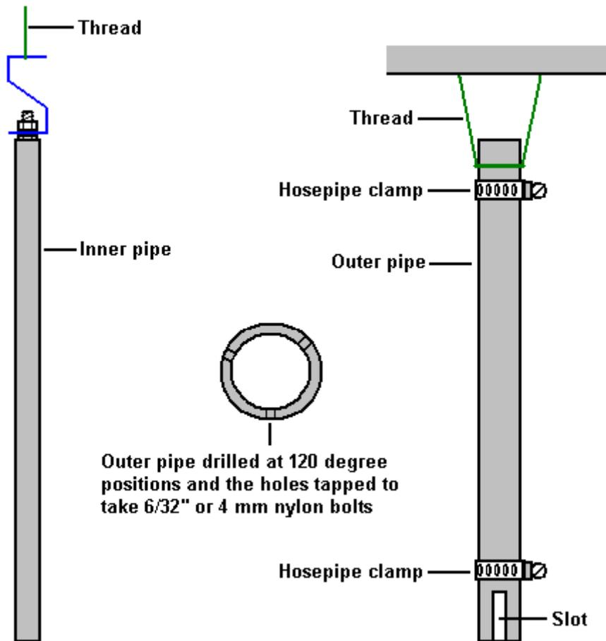
The outer pipes are drilled and tapped to take either a 6/32" nylon bolt available from Ace hardware stores in the USA, or alternatively, drilled and tapped to take a 4 mm nylon bolt. Three of these bolt holes are evenly spaced around the circumference of each end of all of the outer pipes.
