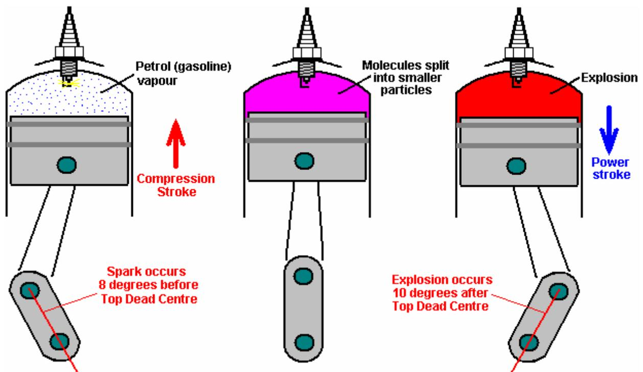
If you were to replace the petrol vapour with hydroxy gas, then there would be a major problem. This is because hydroxy gas has very small molecule sizes which do not need any kind of breaking down and which burn instantly with explosive force. The result would be an explosion which occurs far too soon and which opposes the movement of the rising piston as shown here:
