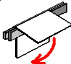
The thickness of the steel bar on the inside of the bend has to be the exact width of the required gap between the finished plate faces. This is not particularly difficult to arrange as 3 mm, 3.5 mm, 4 mm, 5 mm and 6 mm are common thicknesses used in steel fabrication, and they can be combined to give almost any required gap.
