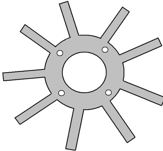
This piece has four holes drilled in it to match the stud positions of the plastic base piece. The number of studs is not specified and while I have shown four, the plate resonance might be helped if there were just three. The size is arranged so that when the arms are bent upwards at right-angles, they fit exactly against the inner face of the acrylic tube.
