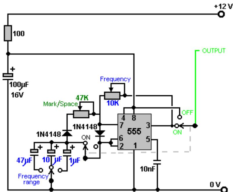
which just has one additional switch to allow the output to be stopped and the 12-volt supply line to be fed instead. The reason for this is that this part of the circuit is used to switch On and Off an identical circuit. This is called "gating" and is explained in Chapter 12 which is an electronics tutorial.
