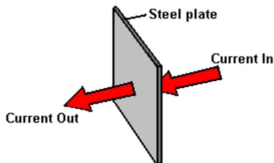
The fact that we have folds and bends in our plates has no significant effect on the current flow. Resistance to current flow through the metal electrode plates is something which can't be overcome easily and economically, and so has to be accepted as an overhead. Generally speaking, the heating from this source is low and not a matter of major concern, but we provide a large amount of plate area to reduce this component of power loss as much as is practical.
