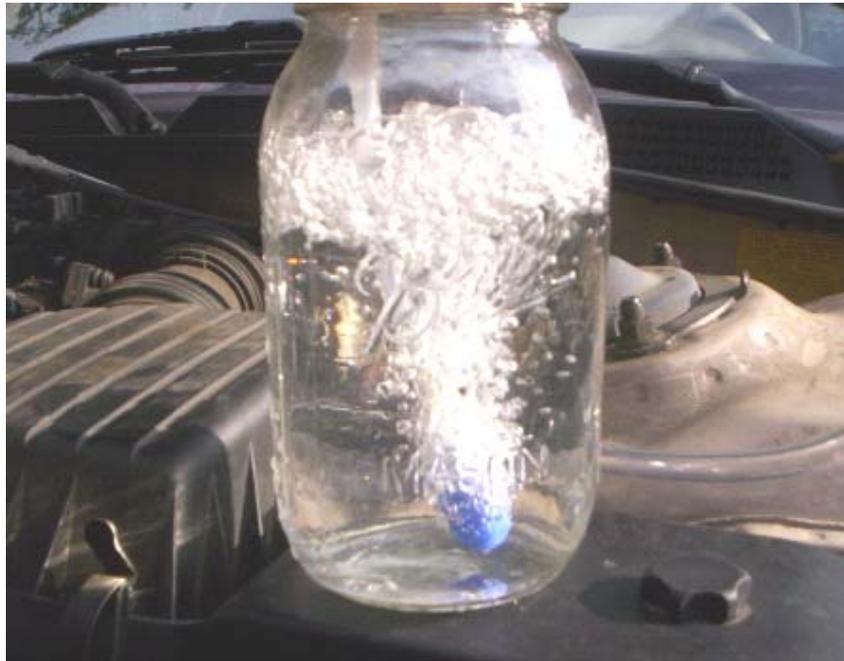
The unit is attached to the air intake of the vehicle, between the air filter and the engine. A small diameter plastic pipe is lead from there to a glass or plastic container holding water. In the above picture Roger is using a glass Mason jar with a screw-on metal lid which has a seal. Sometimes called a preserving jar, these jars are very convenient.
