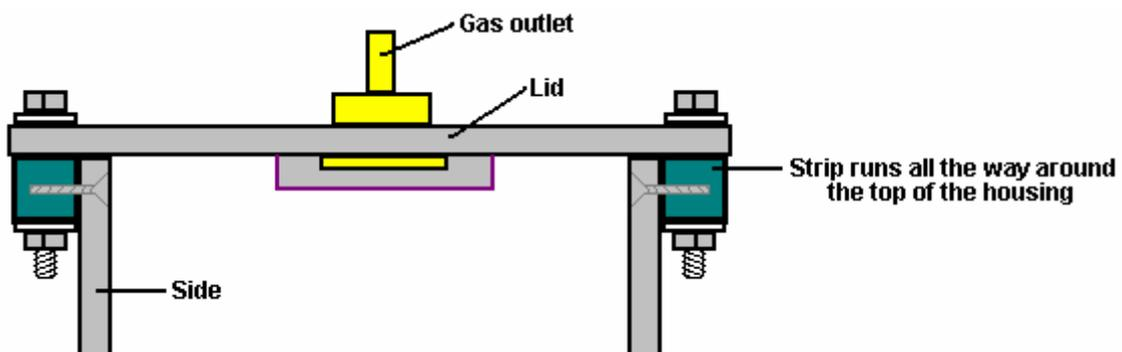
A gasket, perhaps of flexible PVC, placed between the sides and the lid would assist in making a good seal when the lid is bolted down. The gas outlet pipe is located in the centre of the lid which is a position which is not affected if the unit is tilted when the vehicle is on a steep hill.
