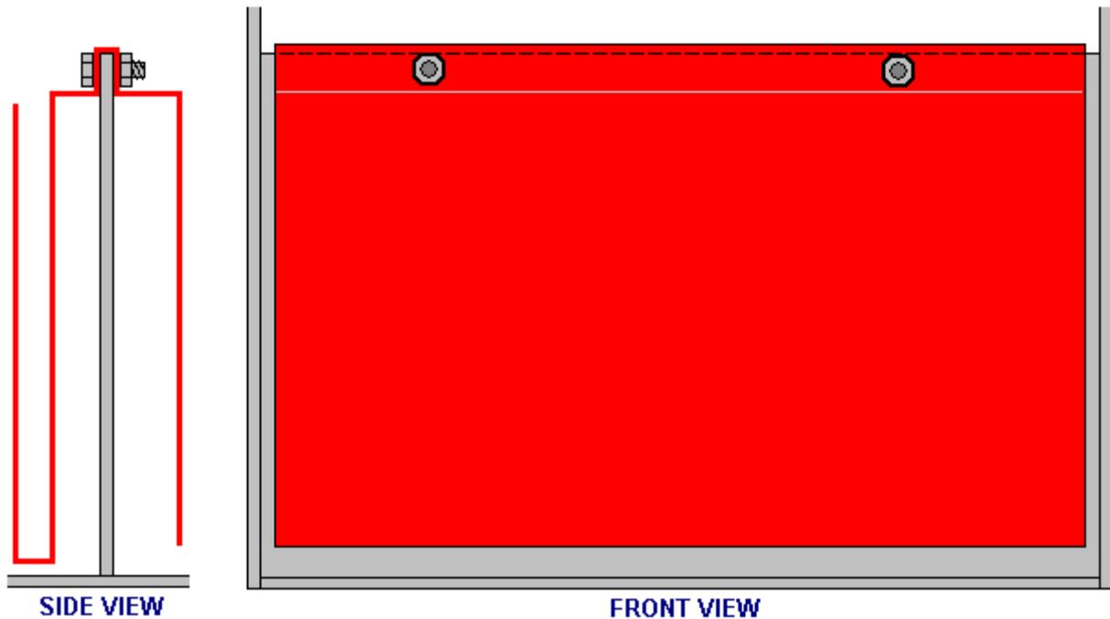
The plate shapes shown above are arranged so that there is access to the bolts from above and they can be reached by a spanner and held steady while the other nut is being tightened.
