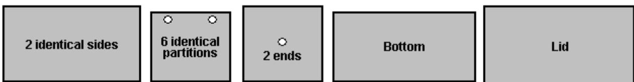
The bottom piece is the same length as the sides, and it is the width of the partitions plus twice the thickness of the material being used to build the housing. If acrylic plastic is being used for the construction, then the supplier can also provide an “adhesive” which effectively “welds” the pieces together making the different pieces appear to have been made from a single piece. The case would be assembled like this:
