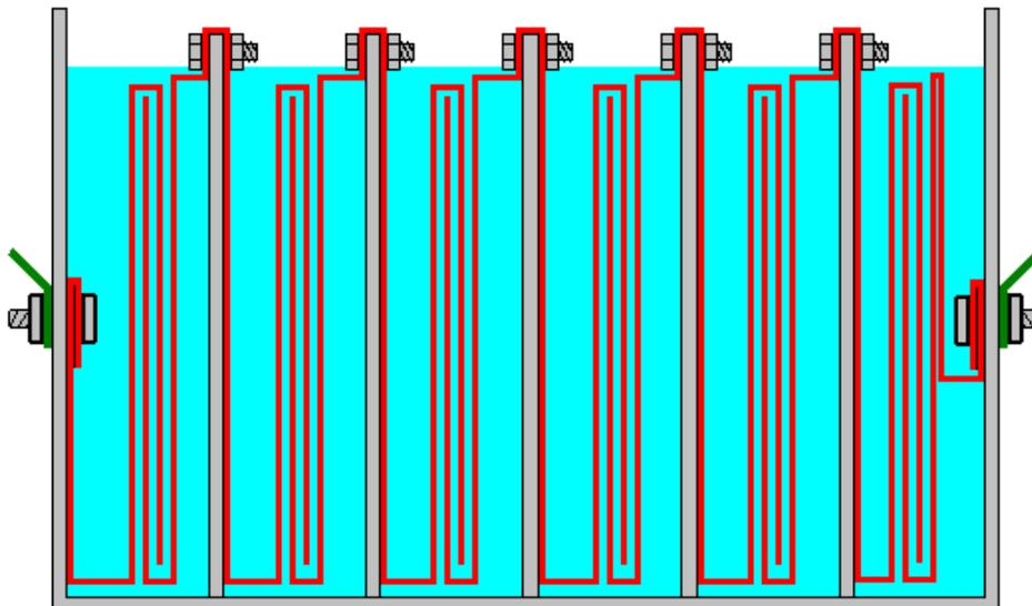
**The electrolyte** is a mix of water and an additive to allow more current to flow through the liquid. Most of the substances which people think of to use to make an electrolyte are most unsuitable, producing dangerous gasses, damaging the surfaces of the plates and giving uneven electrolysis and currents which are difficult to control. These include salt, battery acid and baking soda and I strongly recommend that you do not use any of these.
