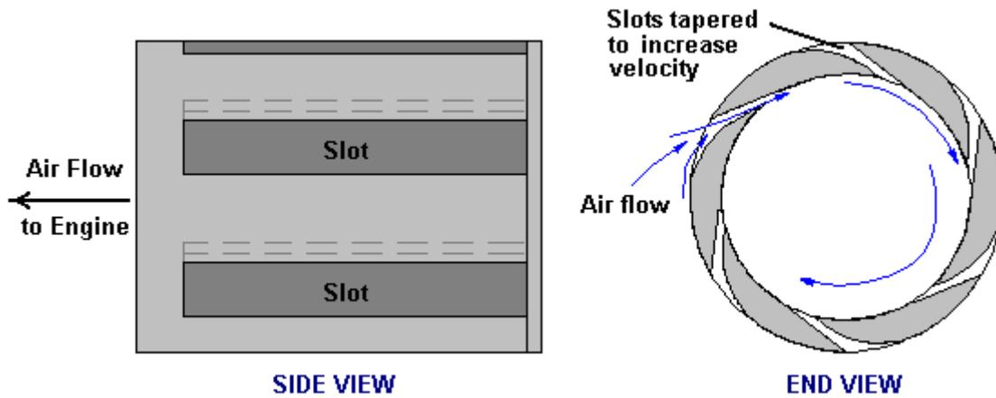
The air enters through each of six tapered slots cut parallel to the axis of the pipe. These give the air an initial spin inside the pipe and the pulsating intake of the engine, combined with the oval shape of the PVC exit T-piece, accelerates the air into a serious vortex which improves the intake to the engine, raising it's efficiency and giving more engine power.
