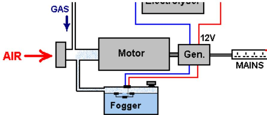
A third method is to use a small carburettor of the type used with model aircraft. This does the same job as a regular engine carburettor, feeding a spray of tiny water droplets into the engine air intake. The physical arrangement of this option depends on the construction of the air filter of the generator being modified.
