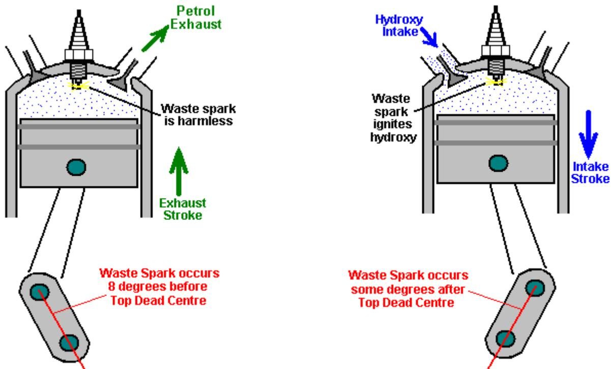
we definitely do not want that to happen, so it is very important that we suppress that additional "waste" spark. So, this leaves us with two engine adjustments: timing delay and waste spark elimination. There are various ways in which these can be done and as each engine design is different, it is difficult to cover every possibility. However, there is a technique which can be used with many engines and which deals with both issues at the same time.
