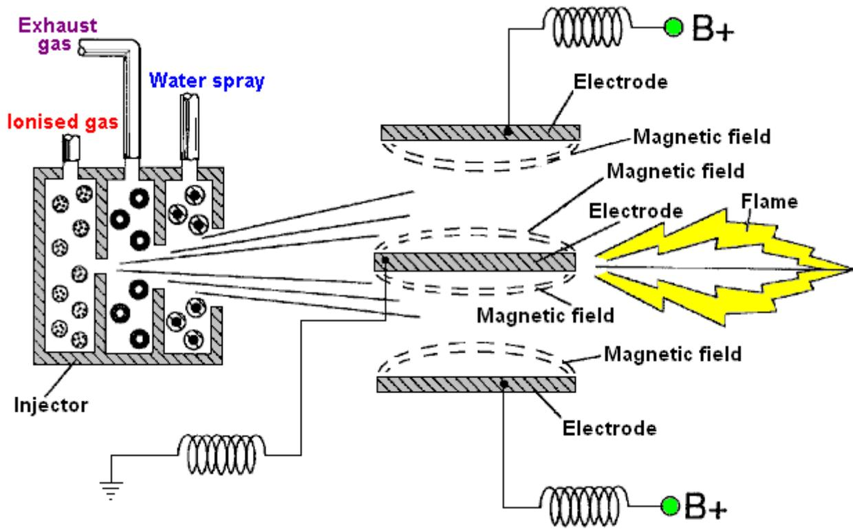
One component is described as ionised gas and ambient air is mentioned. The second component is part of the exhaust gas which is hot water vapour fed through a limiting valve, although inert gases are also mentioned. The third injection component is a very fine spray of water droplets or "mist". This mixture is passed between high voltage electrodes and if the mix does not ignite spontaneously, then it is ignited with a spark.
